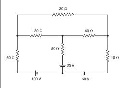
(b) Determine the currents in the various branches of the circuit shown in Figure by nodal analysis?
